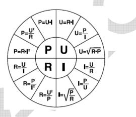
*P* stands for power, *U* for voltage, *R* for resistance and *I* for current. This electrical model has many analogies in other disciplines giving an intuitive sense for physiscs.
