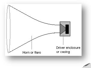
The horn transforms high pressure and low velocity movement from the speaker driver at the horn throat to low pressure and high velocity at the horn mouth by impedance matching.
