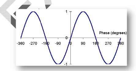
Picture shows a sinewave over two full cycles. The X axis shows the angular relationship but could also be time as frequency =1/t. The Y axis is the level or amplitude.
