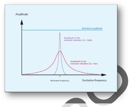
Q is a dimensionless factor in resonance where a high Q means the peak is high and bandwidth small. Even though incorrect use, Q is used for instance to describe the type of roll-off in a reflex speaker. Often the designer chooses the Q such that a pronounced gain occurs just before response rolls of. This accounts for the false impression of low bass found in such designs
