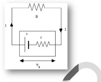
If you apply OHM's law here where P is voltage multiplied by current, you will find that when the battery is loaded (R in the picture) by something with a resistance equaling the battery Ri, maximum power is produced. Note POWER, not current and not voltage, but the product of the two is at its peak when source and destination R's are equal matches.
