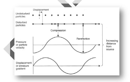
In the two pictures above and below (courtesy John Watkinson, "The art of sound reproduction") we may see the relationship between pressure and velocity of sound. Also seen is how the slope is a function of frequency and amplitude and why larger drivers are required for lower frequencies
